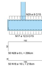
SAPATA - ARMADURAS - CORTE HH
