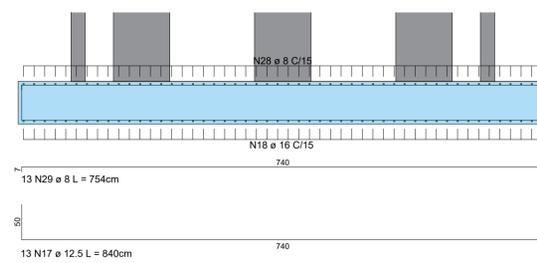
SAPATA - ARMADURAS - CORTE GG
